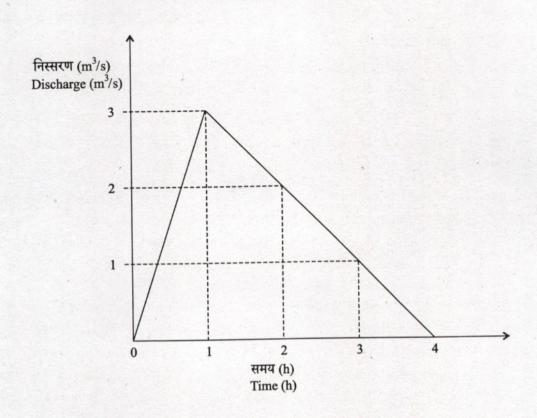
A one-hour unit hydrograph of a catchment is shown in the figure. A storm of two hours duration with intensity of 70 mm/h in the first hour and 40 mm/h in the second hour occurs over the catchment. Calculate the peak direct surface runoff value in m<sup>3</sup>/s.
