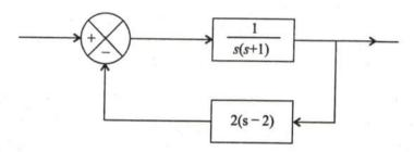
State Nyquist stability criterion. Is the feedback system shown in figure in open loop stable? Determine the closed loop stability of the system using Nyquist stability criterion. Show all the required plots clearly.
