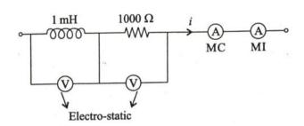
A current of  $(0.5 + 0.3 \sin \omega t - 0.2 \sin 2\omega t)$  amps is passed through the circuit shown in figure. Determine the reading of each instrument if  $\omega = 10^6$  rad/sec.
