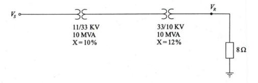
A single phase, single line diagram of a power system is shown in figure. Find the sending end voltage and the value of load resistance in p.u. referred to sending end if the voltage across load resistance is 9.8 KV.
