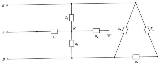
Draw the sequence networks and calculate the load sequence impedances of a load circuit as shown in figure. The load circuit is connected to a balanced three phase supply. The value of  $z_1$ ,  $z_2$  and  $z_n$  are  $(4+j6) \Omega$ ,  $-j45 \Omega$  and  $j4 \Omega$ .
