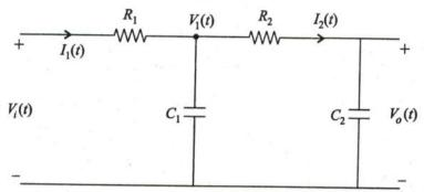
For the network shown in figure, draw a block diagram representing each circuit element by a block. Use block diagram reduction technique to obtain the transfer function of the network. The voltage  $V_i(t)$  is the applied input and the voltage across the capacitor  $V_o(t)$  is the output.
