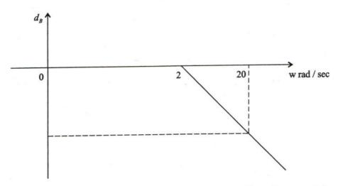
The approximate magnitude plot, obtained experimentally, of a nonminimum phase system is shown in figure. Calculate the phase in degrees at w = 3 rad/sec. 10
