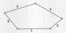
A five-bar chain is shown in the figure. Prove that it is an unconstrained chain.
