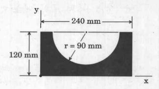
Determine the moment of inertia of the shaded area with respect to the x-axis.
