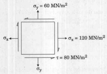
At a certain point in a piece of elastic material, there are normal tensile stresses of magnitude 120 MN/m<sup>2</sup>, 60 MN/m<sup>2</sup> acting orthogonally to each other. In addition, there is a shearing stress of 80 MN/m<sup>2</sup> acting normal to the normal stresses.
