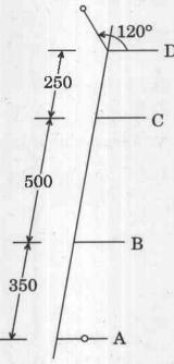
A rotor is completely balanced when masses of 2 kg and 1.2 kg are added temporarily in planes A and D each at 200 mm radius as shown in the figure. The balanced mass in the plane A is along the x-axis whereas in the plane D, it is at 120 mm radius. Determine the magnitudes and the directions of the masses B and C.
