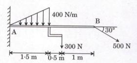
What is the supporting force system at A for the cantilever beam shown in the figure? Neglect the weight of the beam.
