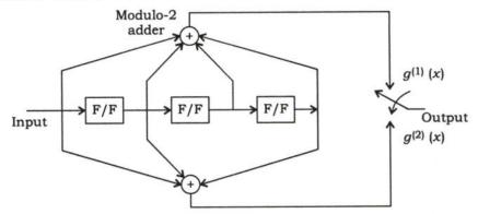
(i) Determine the encoder output produced by the message sequence 11011 ....
