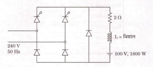
A half-controlled converter fed from 240 V, 50 Hz single-phase ac source is feeding 1800 W power to a 100 V battery as shown in the figure below. The battery is connected in series with a large inductance and a resistance of 2  $\Omega$ . The inductance is large enough to make the load current flat and continuous.
