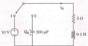
In the series RLC circuit shown in the figure, the capacitor has an initial charge  $Q_0=1\,$  mC and the switch is in position 1 long enough to establish the steady state. Find the transient current which results when the switch is moved from position 1 to 2 at t = 0.
