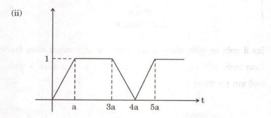
Obtain the Laplace transform of the following periodic waveforms:
