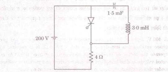
The circuit given in the figure below is in steady state initially before the thyristor is triggered. The thyristor is triggered at t = 0. Calculate
