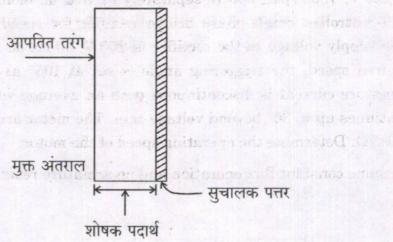
An absorber material of relative permeability and relative permittivity of  $\epsilon_r = \mu_r = 6$  – j6 is coated on a perfectly conducting sheet and this combination is placed in free space as shown in the figure given below. A 500 MHz wave is incident on it normally from free space. Calculate the thickness of the absorber required to attenuate the reflected wave by 30 dB.
