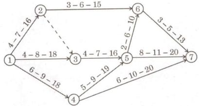
The network for a construction project is shown in the figure given below. The three time estimates for each activity are given along each activity arrow. Determine the:
