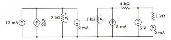
In the circuit given here, find the value of voltage  $v_1$ :
