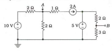
Find the voltage on points A and B of the given circuit:
