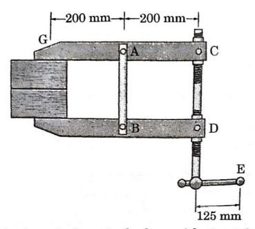
A gripper is shown in the figure. A horizontal force F=50~N is applied to the handle of the lever at E. The mean diameter of the single square threaded screw at C and E is 25 mm and lead is 5 mm. Determine the clamping force developed at G. The coefficient of static friction is  $\mu_S=0.3$ .
