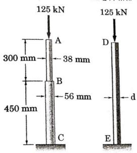
The aluminium rod ABC having Young's modulus 70 GPa consisting of two cylindrical portions AB and BC, is to be replaced with a cylindrical steel rod DE with Young's modulus 200 GPa of same overall length. Determine minimum required diameter, d, of the steel rod if its vertical deformation is not to exceed the deformation of aluminium rod under the same load and if the allowable stress in the steel rod is not to exceed 165 MPa.
