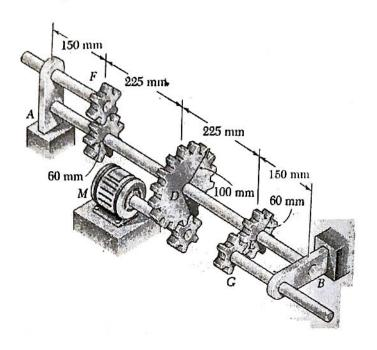
A solid shaft AB rotates at 450 rpm and transmits 20 kW from the motor M to machine tools connected to gears F and G. A power of 8 kW is taken off at gear F and 12 kW is taken off at gear G. The allowable shear stress is 55 MPa. Determine the smallest permissible diameter of the shaft AB.
