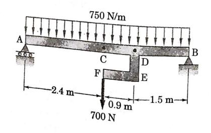
A beam AB under loading is shown in the figure. The rigid bar DEF is welded at a point D. The Young's modulus of the beam material is 200 GPa and its moment of inertia is  $20 \times 10^6$  mm<sup>4</sup>.
